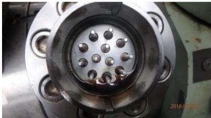
Liquid migration within connectors (sensor/power)
