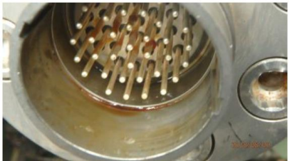
Liquid migration within connectors (sensor/power)
