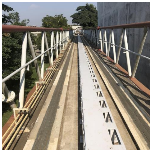
Figure 3 The new Induction Motor 200 meters long secondary made with Aluminium sheets and back iron.
