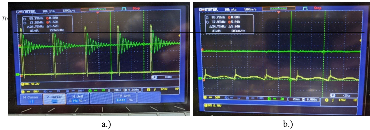
Figure 8. Measured voltage (yellow) and current (green) on the output of the amplifier without the filter (a) and with the filter (b). The DC output current component was 5.52A without the filter and 5.04A with the filter.
