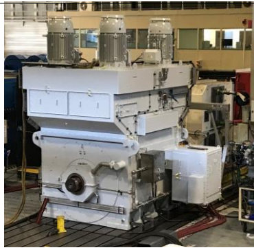
Figure 30 Rotor heat test arrangement (16MW Motor side).
