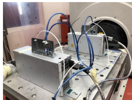
Figure 27 Assembly on vibration machine.
