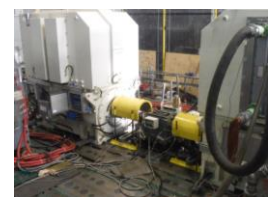
Figure 19 Back-to-back test arrangement.
