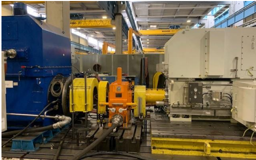
Figure 20 Load test with gearbox (high-speed motor on the right)
