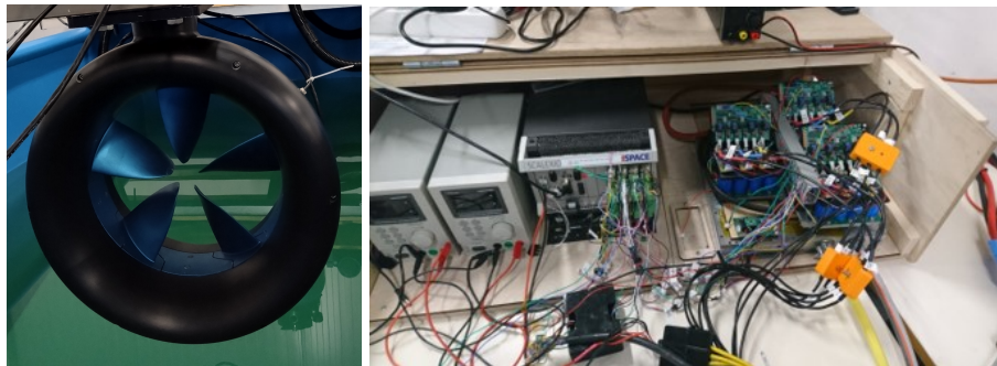
Figure 5: 20 kW hubless rim-driven thruster and control setup
