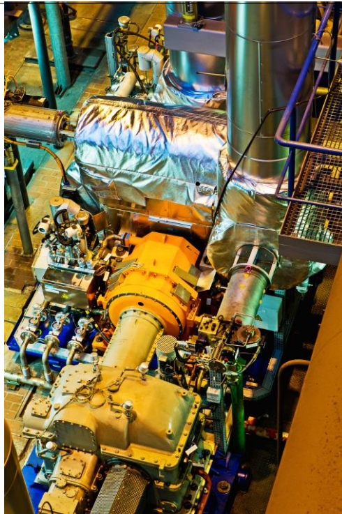
Figure 2 SPAT prototype in the Jaenschwalde powerplant. The orange bearing housing is identical in construction to the SFDT
