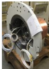
Figure 8 Active magnetic bearing integration for easy maintenance.
