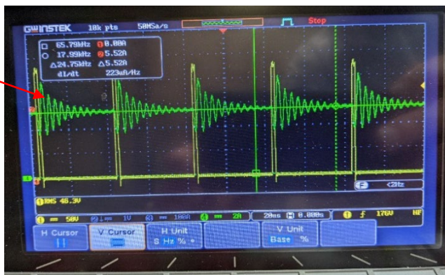
Without filter, I_{out}=5.52A
